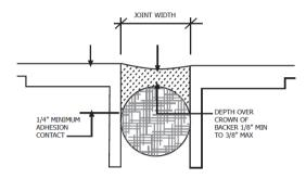
The sealing joint gap is formed using a sealant-compatible backer foam, which supports the sealant during application and provides a bond breaker at the base of the slot to allow movement to be accommodated over the full width of the sealant.
